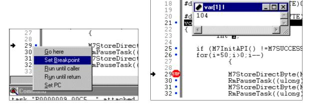
**Tip** Breakpoints can be set only on lines which are marked with a blue dot following the line number.
