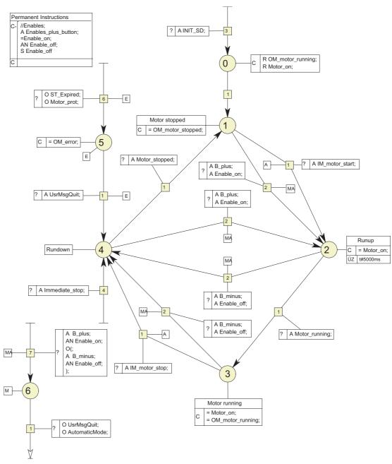
In our example we are going to use the state graph both for controlling the motor and the coolant, that is, we need to create two instances.
