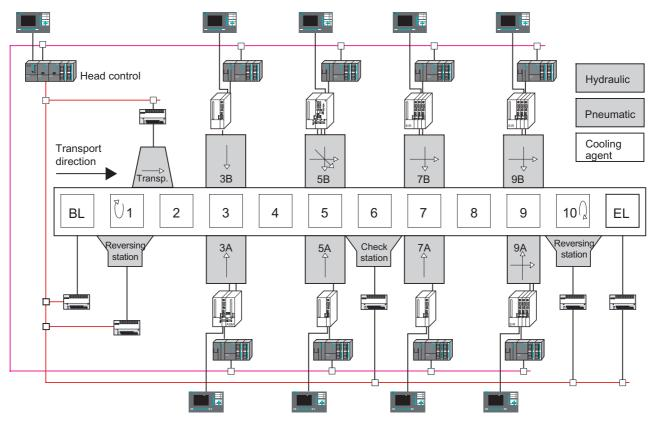
Each processing unit is usually assigned a control system with operator panel. Each unit is equipped with 1 to 4 controlled drives (axes / spindles), for which we require single-axis modules or NCs (SINUMERIK 810D/840D, for example.)
