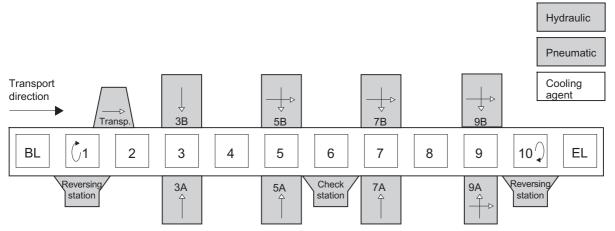
The stations 1 to 10 are assigned to processing units (3A, 3B, 5A, etc.), reversing stations (1, 10) or inspection stations (6). The line starts at the delivery point DEP, and ends at the discharge point DIP The media supply (coolants, hydraulic and pneumatic system) is controlled in higher-ranking operations. One of the processing units used by the drill unit.
