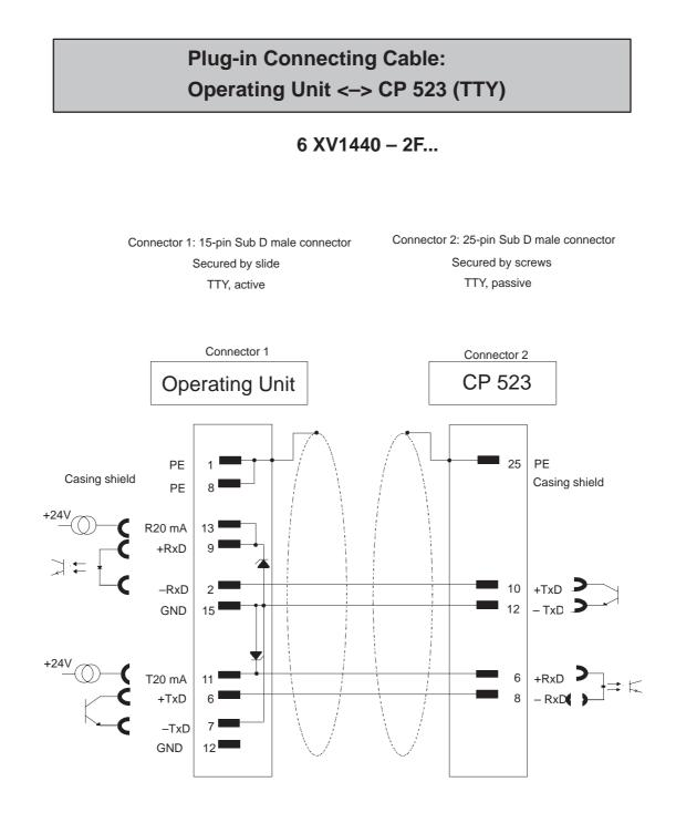
For TTY cables with special lengths > 10m, 2 Zener diodes (12 V) must be soldered in the 15-pin connector for the operating unit (TTY active): BZX 55 C12 ser. no. 30095128
