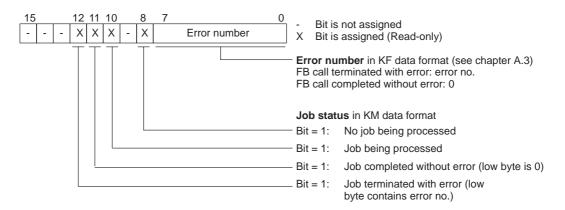
Figure 5-2 Contents of AKKU 1 after Invoking Standard FB
