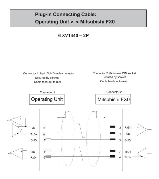
Cable: 3 x 2 x 0.14 mm<sup>2</sup>; shielded; max. length 500 m Shielding connected at both ends to casing with large contact area
