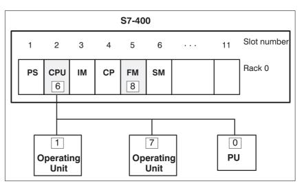
Figure 12-6 Network Configuration with S7-400 and Operating Unit – one Rack
