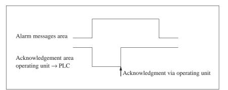
Figure 11-5 Signal Diagram for Acknowledgement Area Operating Unit  $\rightarrow$  PLC
