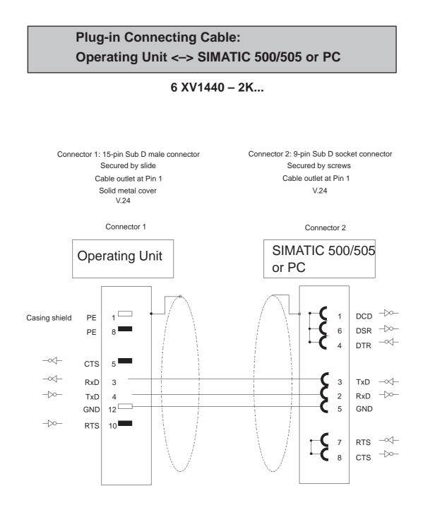
Shielding connected at both ends to casing with large contact area Cable:  $5 \times 0.14 \text{ mm}^2$ ; shielded; max. length 15 m
