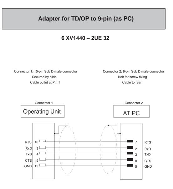
Cable: 5 x 0.14 mm<sup>2</sup>; shielded; max. length 32 cm Shielding connected at both ends to casing with large contact area
