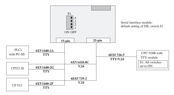
Figure C-1 Positions of the switch elements; default setting
