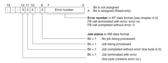
Figure 10-2 Contents of AKKU 1 after Invoking Standard FB
