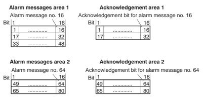
Figure 17-3 Assignment of Acknowledgement Bit and Message Number
