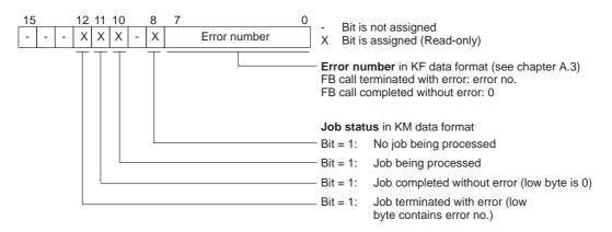
Figure 4-2 Contents of AKKU 1 after Invoking Standard FB
