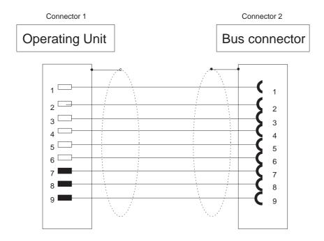
Cable: 9 x 0.14 mm2, shielded; length 5 cm Shielding connected at both ends to casing with large contact area Installation of multiple OP15s one under another (e.g. 3x6 = 18 units at intervals of 3 cm) 6XV1440-2TE10 can not be used.
