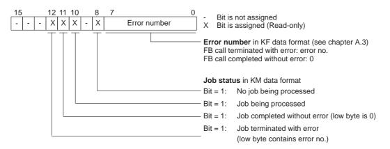
Figure 4-4 Contents of AKKU 1 after Invoking Standard FB
