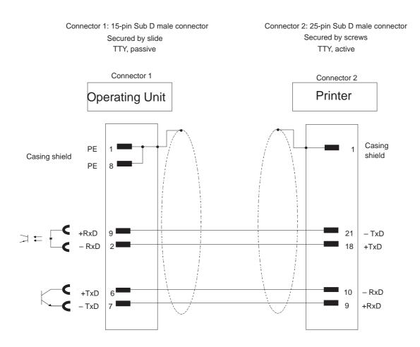
Cable: 5 x 0.14 mm<sup>2</sup>; shielded; max. length 1000 m Shielding connected at both ends to casing with large contact area
