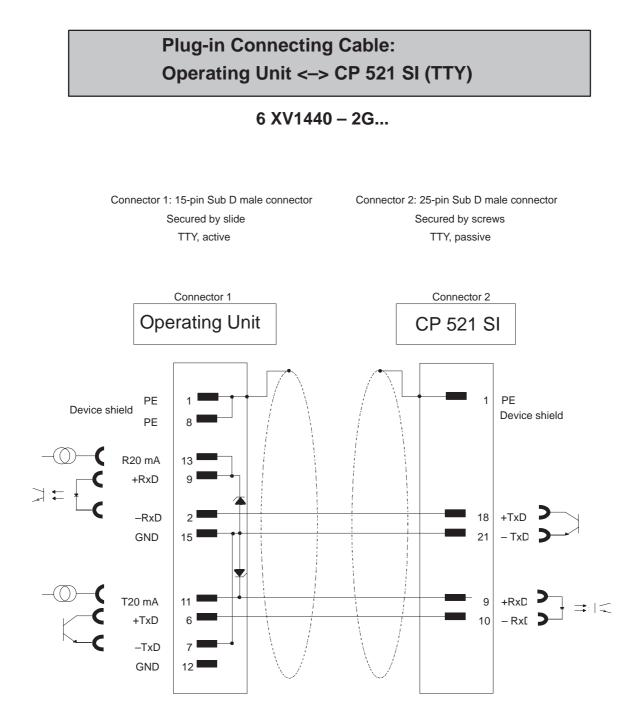
For TTY cables with special lengths > 10m, 2 Zener diodes (12 V) must be soldered in the 15-pin connector for the operating unit (TTY active): BZX 55 C12 ser. no. 30095128
