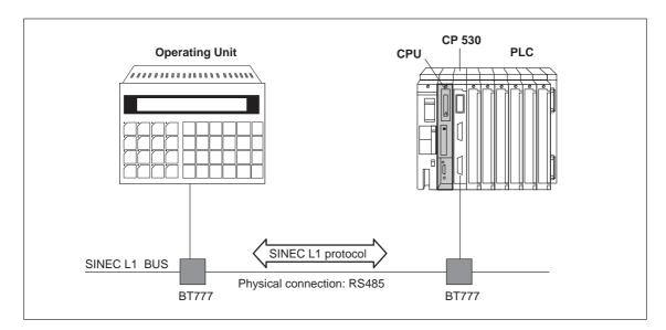
Figure 1-4 SINEC L1 Connection
