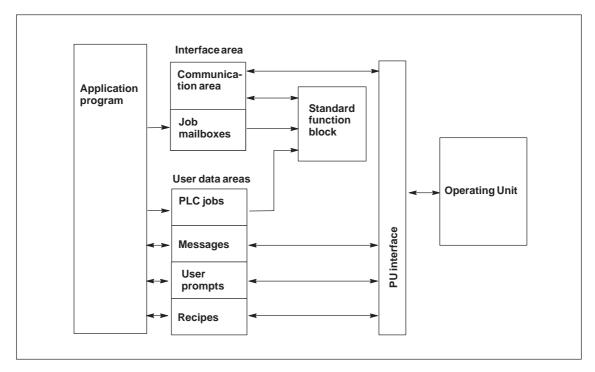
Figure 3-1 AS511 Communication Structure for Group 2 PLCs
