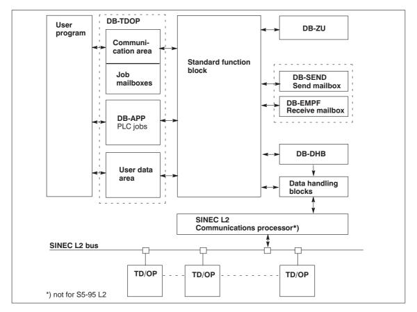
Figure 8-1 Communication structure of the SINEC L2 connection
