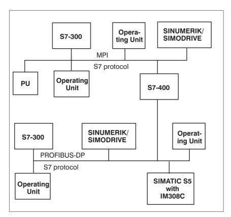
Figure 12-1 S7 network configurations
