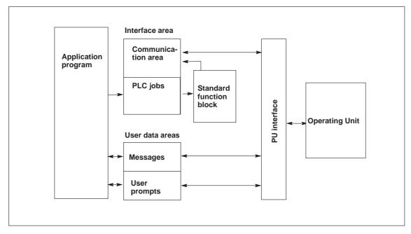
Figure 4-1 AS511 Communication Structure for Group 1 PLCs
