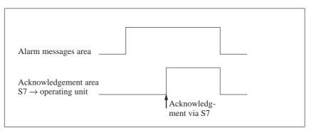
Figure 14-4 Signal Diagram for Acknowledgement Area  $S7 \rightarrow Operating Unit$
