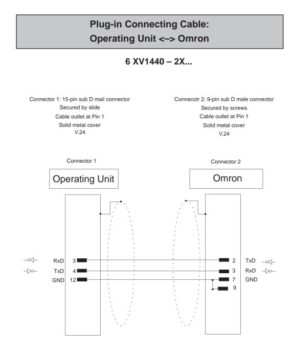
Shielding connected to casing with large contact area Cable:  $5 \times 0,14$ mm<sup>2</sup>; shielded; max. length 15m
