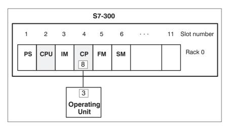
Figure 12-9 Network Configuration with S7-300 and Operating Unit – PROFIBUS-DP Profile
