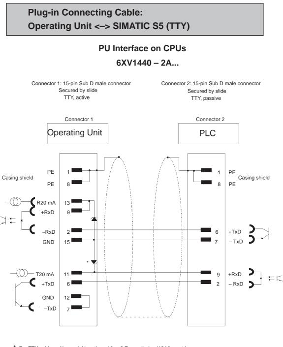
\* For TTY cables with special lengths > 10m, 2 Zener diodes (12 V) must be soldered in the 15-pin connector for the operating unit (TTY active):
