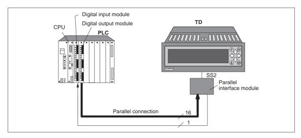
Figure 9-1 Parallel connection: standard configuration
