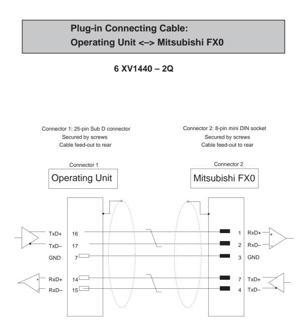
Cable:  $3 \times 2 \times 0.14 \text{ mm}^2$ ; max. length 500 m Shielding connected at both ends to casing with large contact area
