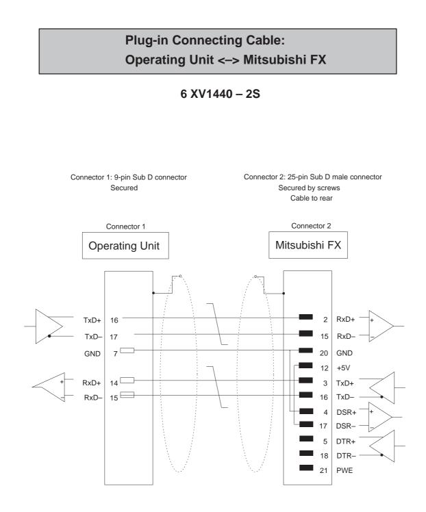
Cable:  $3 \times 2 \times 0.14 \text{ mm}^2$ ; max. length 500 m Shielding connected at both ends to casing with large contact area
