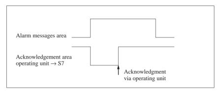
Figure 14-5 Signal Diagram for Acknowledgement Area Operating Unit  $\rightarrow$  S7
