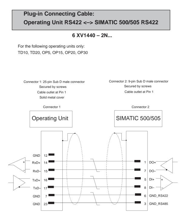
Shielding connected to casing with large contact area Cable: 3 x 2 x 0.14 shielded; max. length 300 m  $\,$
