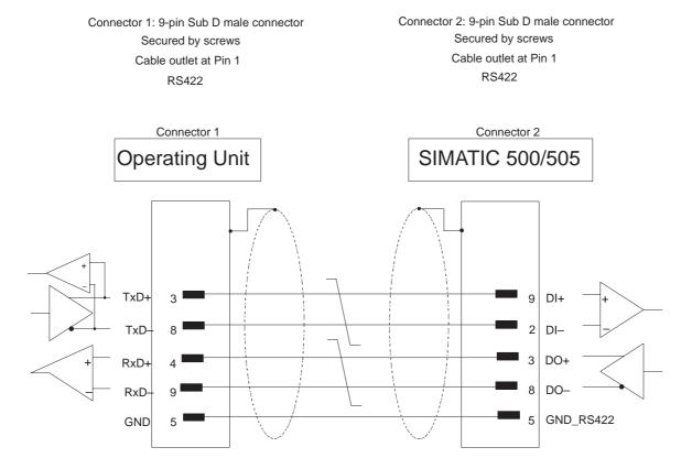
Shielding connected to casing with large contact area Cable: 3 x 2 x 0.14 mm²; shielded; max. length 300 m  $\,$
