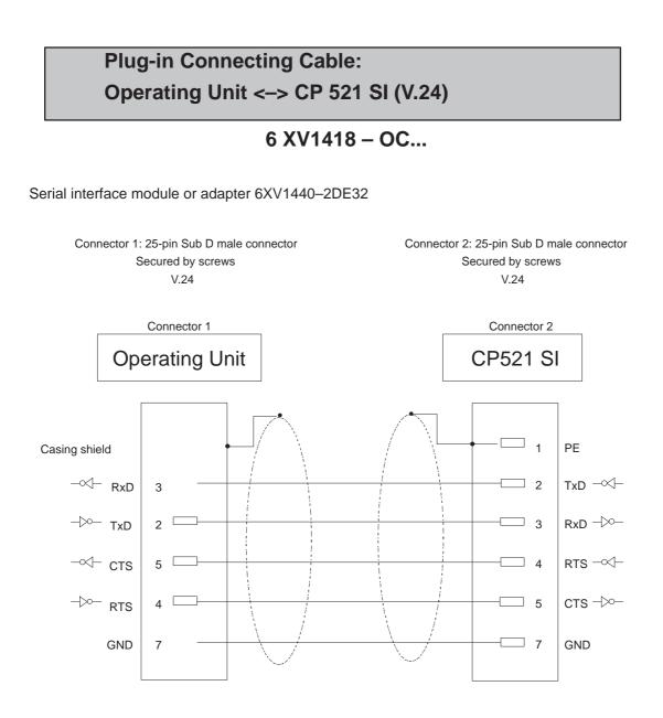
Cable: 5 x 0.14 mm<sup>2</sup>; shielded; max. length 15 m Shielding connected at both ends to casing with large contact area
