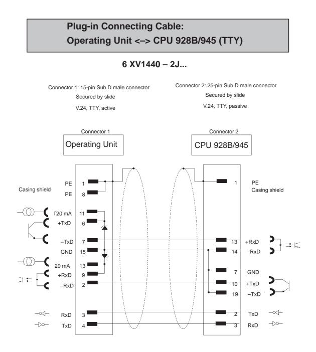
Cable: 5 x 0.14 mm<sup>2</sup>; shielded; max. length 1000 m Shielding connected at both ends to casing with large contact area
