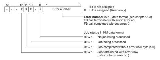
Figure 6-4 Contents of AKKU 1 after Invoking Standard FB
