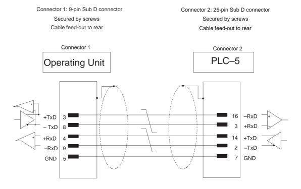
Cable 3 x 2 x 0.14 mm<sup>2</sup>; shielding contacts joined; max. length 60 m Shielding connected at both ends to casing with large contact area
