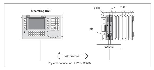
Figure 1-2 Connection using Free ASCII Protocol (FAP)
