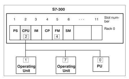
Figure 12-4 Network Configuration with S7-300 and Operating Unit – oneRrack
