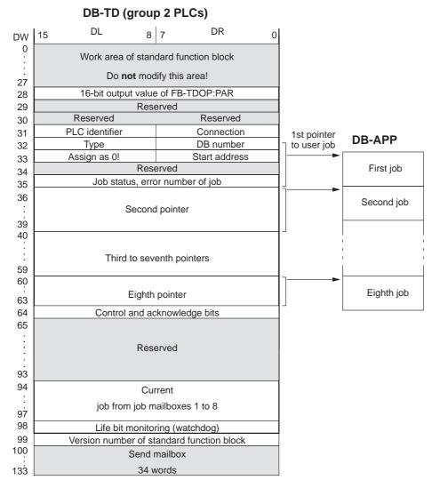
Figure 9-6 Structure of the interface area for group 2 PLCs
