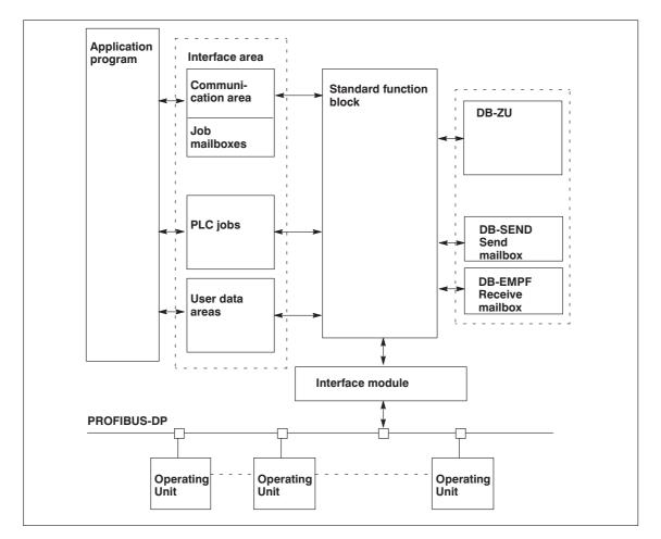
Figure 6-1 Communication Structure for PROFIBUS-DP Connection
