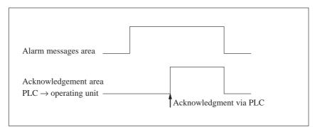
Figure 11-4 Signal Diagram for Acknowledgement Area PLC  $\rightarrow$  Operating Unit
