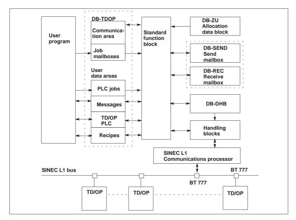
Figure 7-1 Communication structure of the SINEC L1 connection
