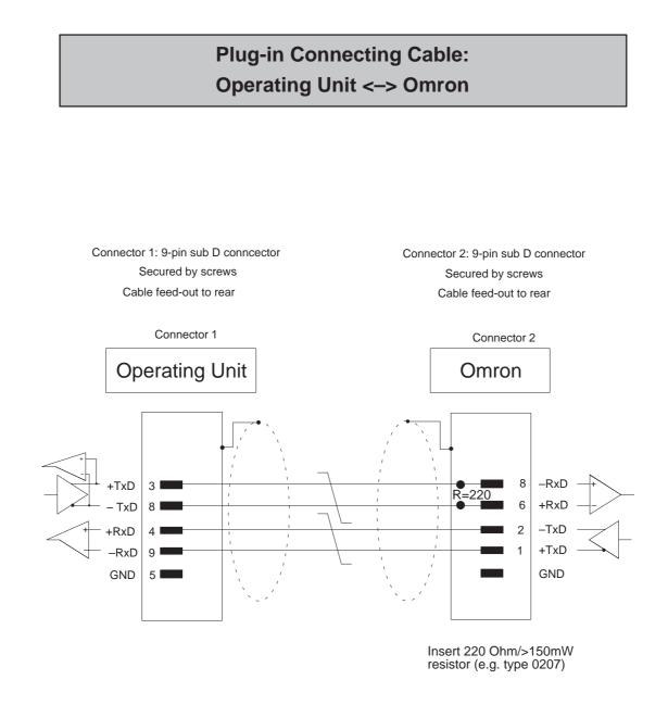
Cable: 3 x 2 x 0,14mm<sup>2</sup>; shielding contacts joined; max. length 500 m
