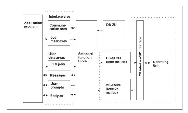
Figure 5-1 Communication Structure for FAP Connection
