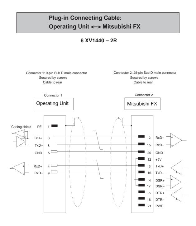
Cable:  $3 \times 2 \times 0.14 \text{ mm}^2$ ; max. length 500 m Shielding connected at both ends to casing with large contact area
