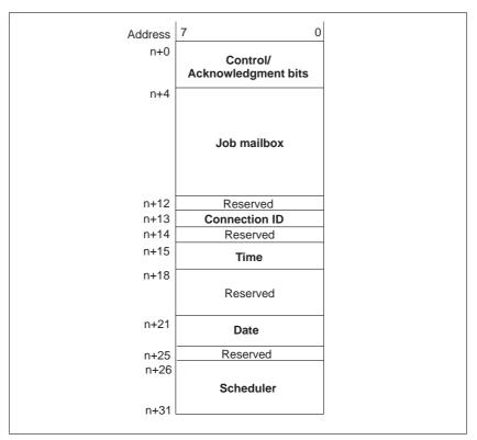
Figure 13-1 Layout of interface area for SIMATIC S7
