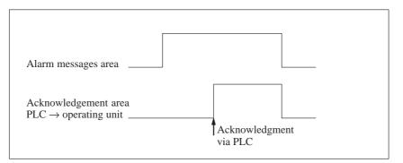
Figure 17-4 Signal Diagram for Acknowledgement Area PLC  $\rightarrow$  Operating Unit
