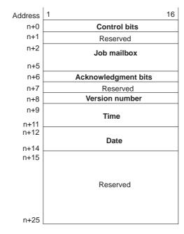
n = Address of configured *user data type* Figure 16-1 Layout of Interface Area for SIMATIC 500/505
