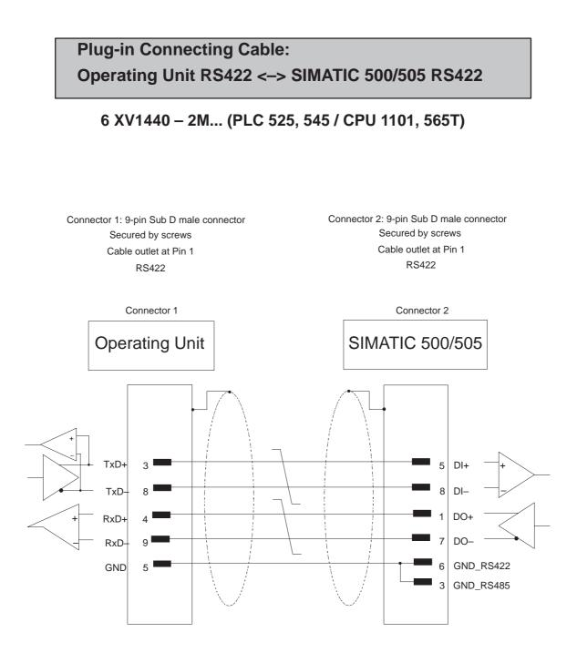
Shielding connected to casing with large contact area Cable:  $3 \times 2 \times 0.14 \text{ mm}^2$ ; shielded; max. length 300 m
