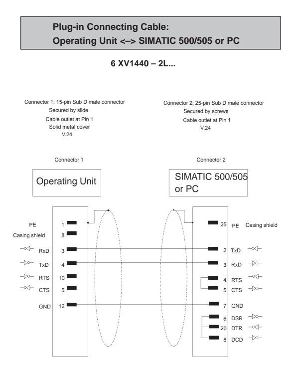
Shielding connected to casing with large contact area Cable:  $5 \times 0.14 \text{ mm}^2$ ; shielded; max. length 15 m
