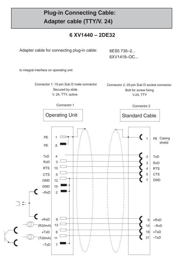
Cable: 9 x 0.14 mm<sup>2</sup>; shielded; max. length 0.3 m Shielding connected at both ends to casing with large contact area
