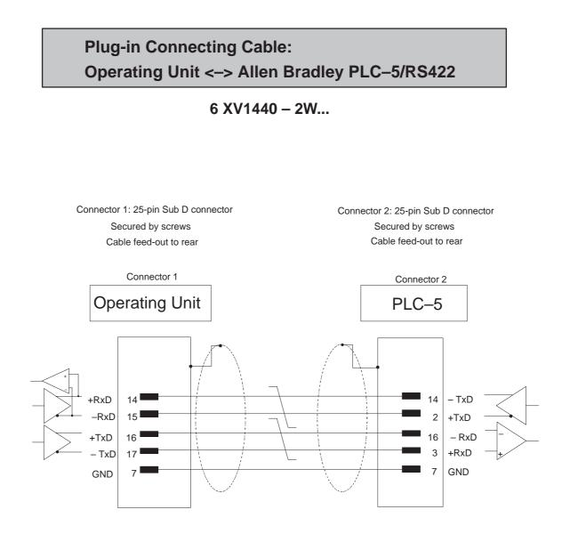
Cable 3 x 2 x 0.14 mm<sup>2</sup>; shielded; max. length 60 m Shielding connected at both ends to casing with large contact area Shielding contacts joined.
