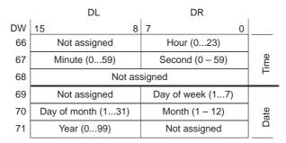
Figure 10-3 Layout of Data Area for Time and Date
