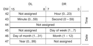
Figure 4-5 Layout of data area for **Time** and **Date**
