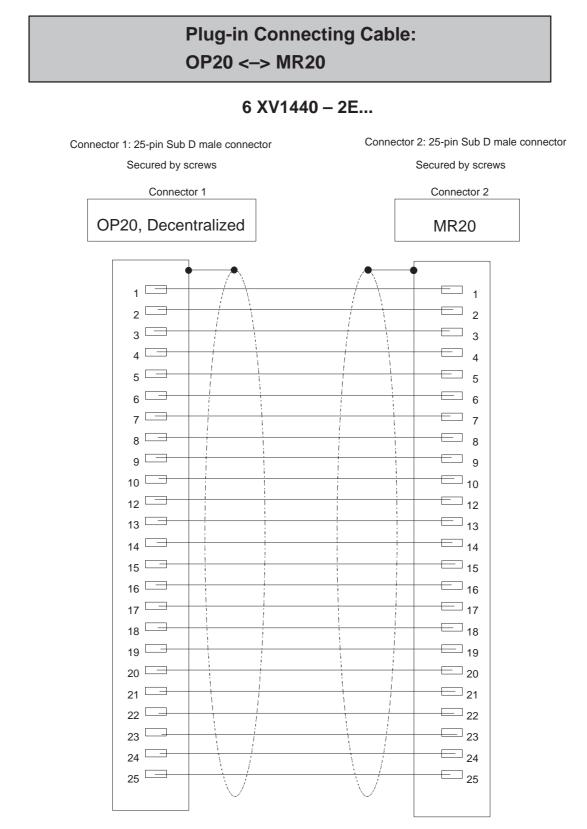
Cable 26 x 0.18 mm<sup>2</sup>; shielded; max. length 3.2 m Shielding connected at both ends to casing with large contact area
