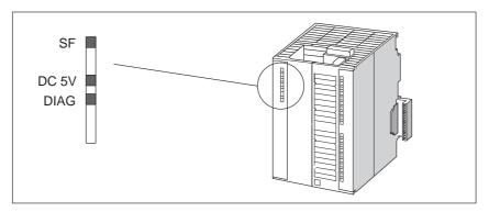
Fig. 11-2 Status and error displays of the FM 353
