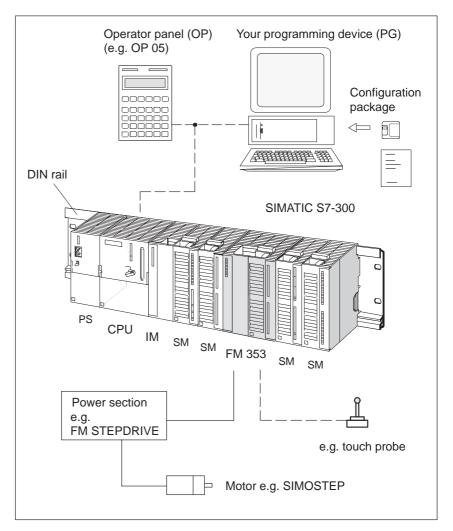
Fig. 1-2 System overview (schematic)
