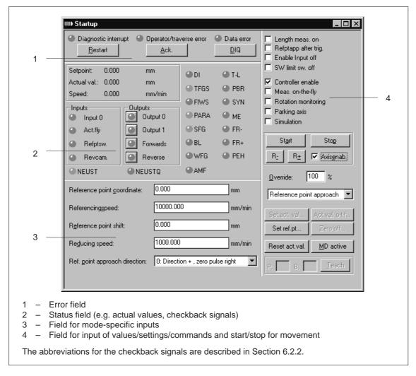
Fig. 7-2 Startup interface (e.g. for "Reference-point approach" mode)
