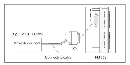
Fig. 4-5 Connecting a drive unit
