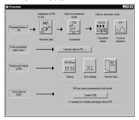
Fig. 7-1 Overview display for parameterization and start-up
