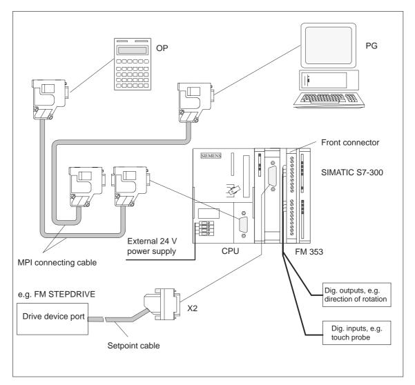
Fig. 4-1 Wiring an FM 353
