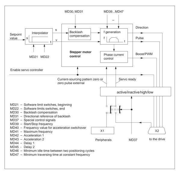
Fig. 9-6 Overview of stepper motor control system
