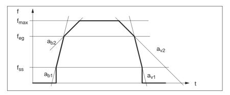
Fig. 9-7 Maximum speed frequency profile
