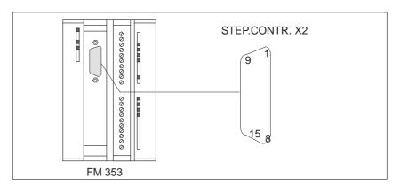
Fig. 4-2 Position of X2 connector
