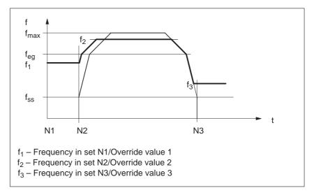
Fig. 9-8 Frequency profile with G64 or speed override
