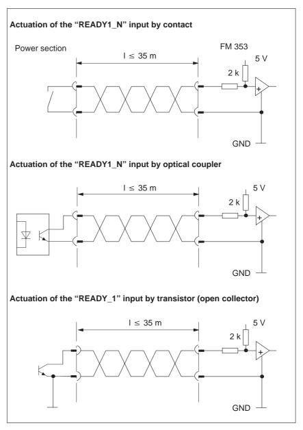
Fig. 4-4 Connection of the "READY1\_N" input
