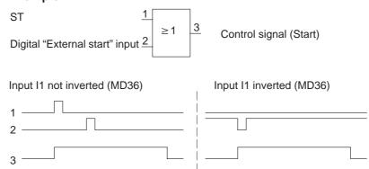
Minimum signal length at the digital input: ≥ 2 · FM cycle
