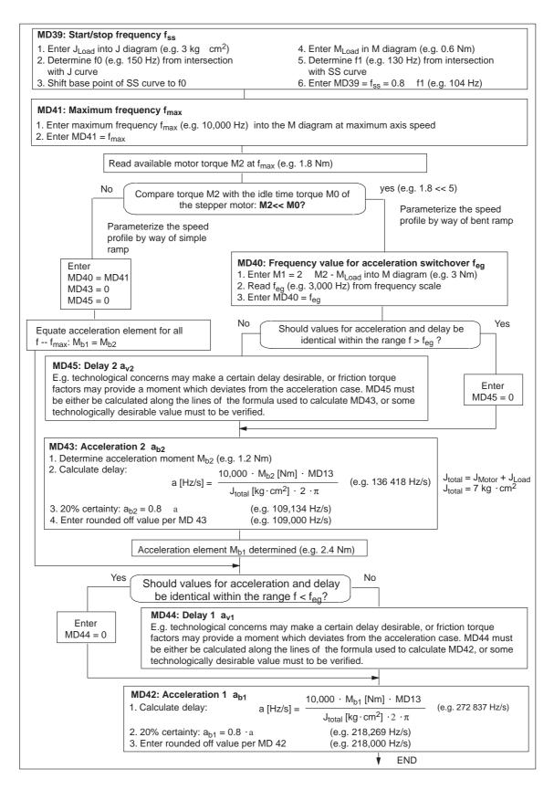
Fig. 7-6 Evaluation of operating characteristic curves
