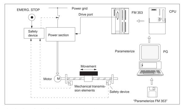
Fig. 2-2 Setup of positioning with stepper motor (example)
