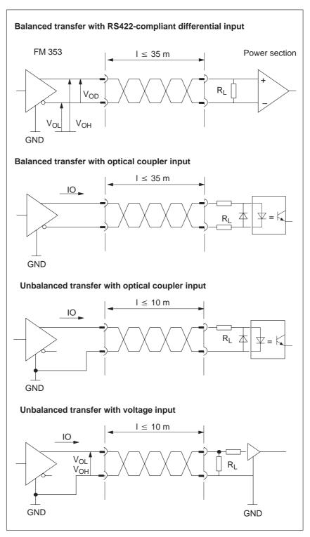
Fig. 4-3 Connection options for drive port output signals.
