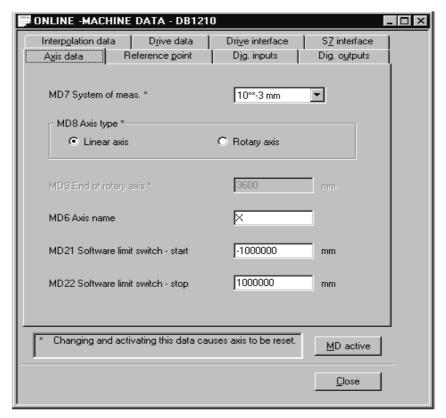
Fig. 5-4 Entering values for machine data
