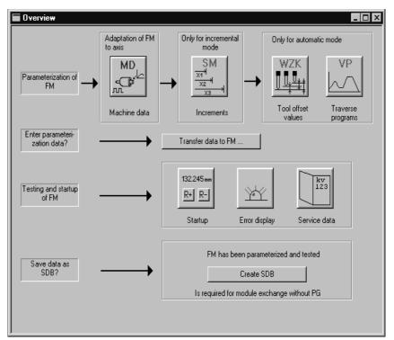
Fig. 5-3 Overview display for parameterization
