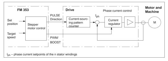
Fig. 7-9 Structure of the stepper motor axis
