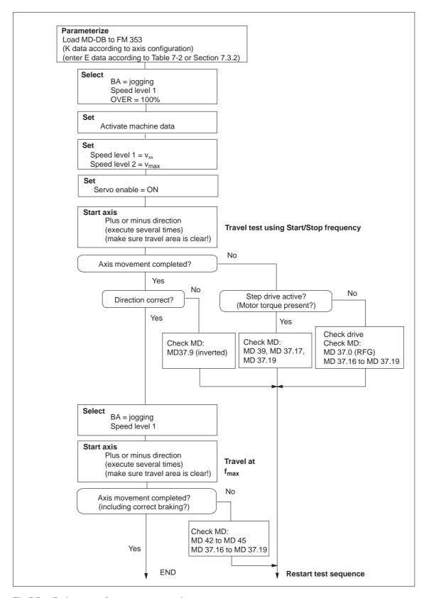
Fig. 7-7 Basic startup of stepper motor control
