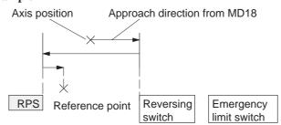
The value for the reference-point shift (MD27) is traveled after the synchronization point is reached.
