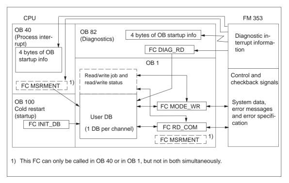
Fig. 6-2 Overview of linking the FM 353 into the user program
