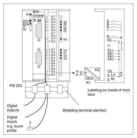
Fig. 4-9 Wiring of the front connector
