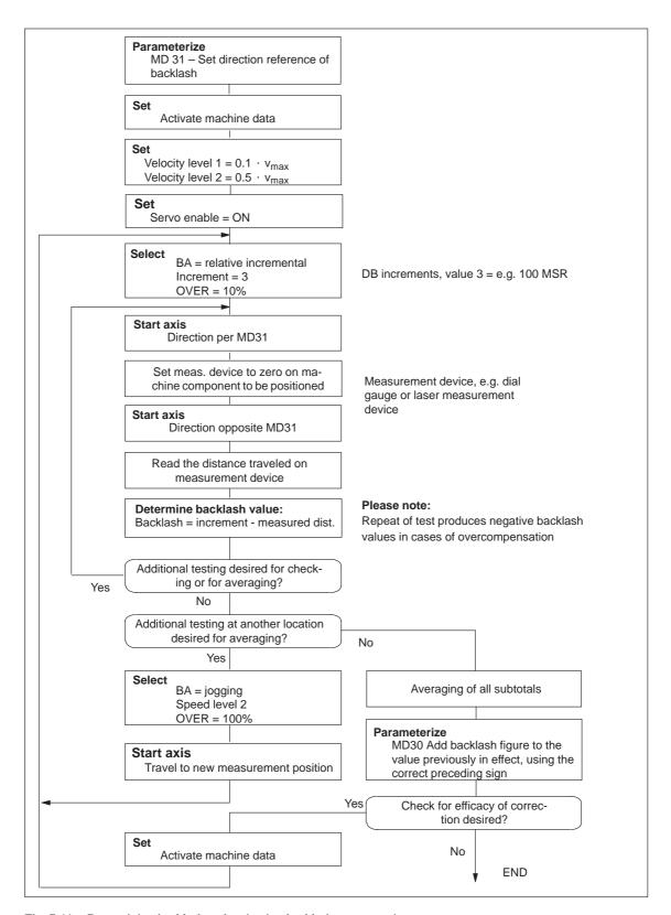
Fig. 7-11 Determining backlash and activating backlash compensation
