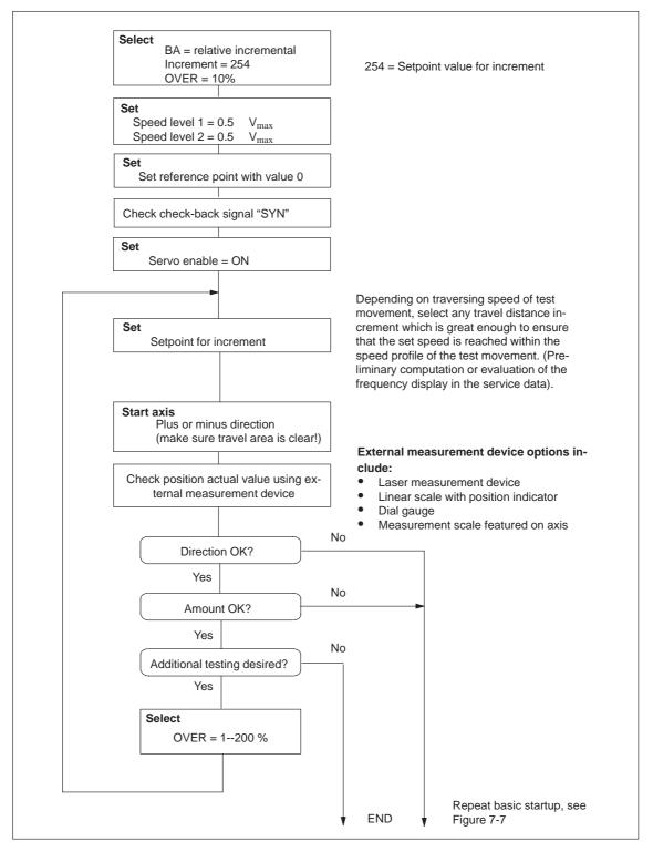
Fig. 7-8 Positioning verification
