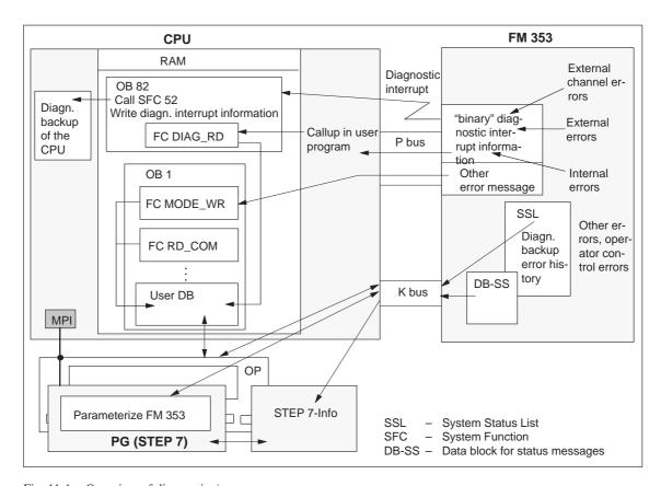
Fig. 11-1 Overview of diagnostics/errors
