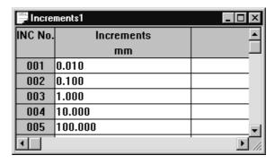
Fig. 5-6 Entering values for incremental dimensions
