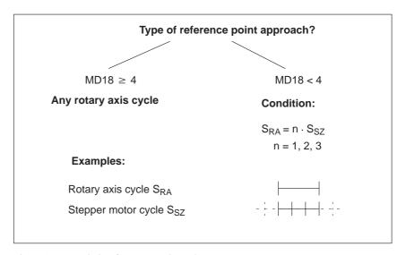
Fig. 9-5 Restriction for rotary axis cycle
