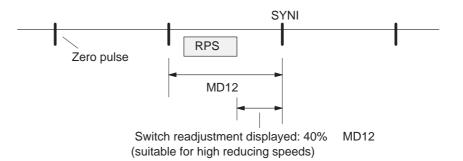
Set the referencing velocity to the highest value compatible with your requirements. It is important for it to be possible to brake to the reducing speed along the entire length of the reference-point switch (RPS). If this is not the case, an additional repositioning to the RPS occurs before the search phase begins. Compare the cycle of the executed traversing movements with Section 9.2.3 and optimize the referencing speed (MD28).
