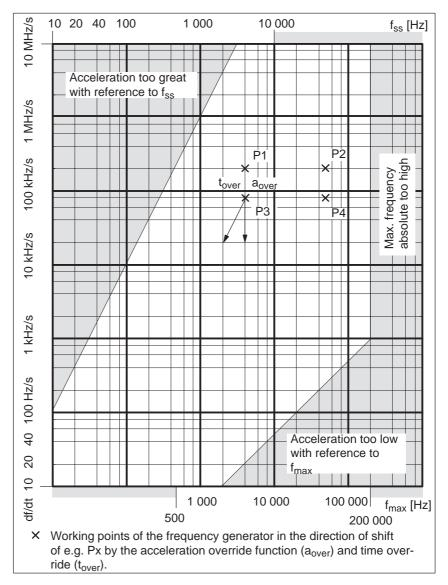
Fig. 5-5 Working range, frequency generator
