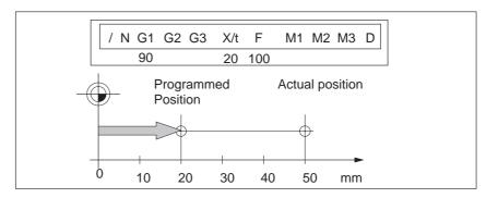
Fig. 10-1 Reference-measure input G90
