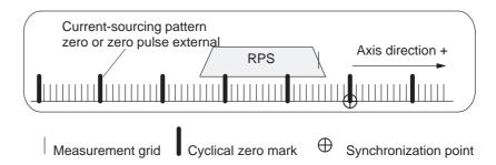
With reference to the synchronization point, the reference point can be located on the side of the lower or the higher position actual values. In the "reference point approach" operating mode the machine axis additionally traverses this distance, during its last phase of motion, once the synchronization point has been found. Consequently, the axis halts the motion, in each instance, exactly on the reference point.
