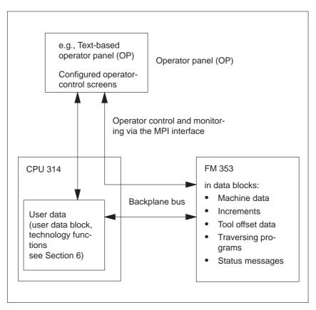
Fig. 8-1 Operator control and monitoring for the FM 353
