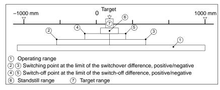
Figure 2-2 Ranges and Switching Points Around the Target
