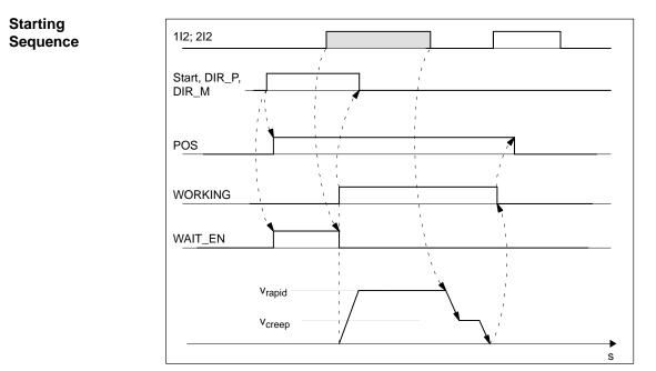
Figure 9-3 Starting the Incremental Mode
