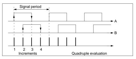
Figure 10-2 Quadruple Evaluation
