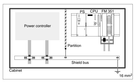
Figure 4-2 Installation in a Cabinet
