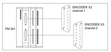
Figure 4-4 Position of the Subminiature Cannon Sockets X2 and X3
