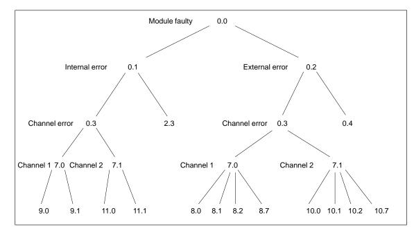
Figure 11-2 Diagnostic Chart: Bits in the Channel DBs from Byte 72 Onwards (DIAGNOSTIC\_INT\_INFO)
