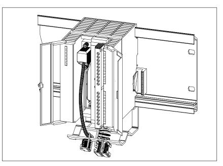
Figure 4-5 Connection of an Encoder to the FM 351 Positioning Function Module
