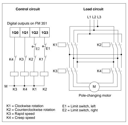
Figure 4-3 Contactor Circuit
