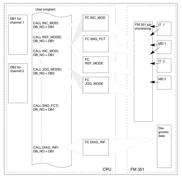
Figure 6-1 Principle of Communication between the CPU and FM 351
