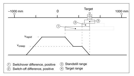
Figure 2-3 Velocity Curve on Approaching a Target Position (Basic Shape)
