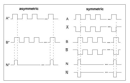
Figure 10-1 Signal Waveforms from Incremental Encoders
