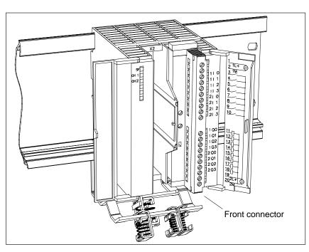
Figure 4-6 Position of the Front Connector
