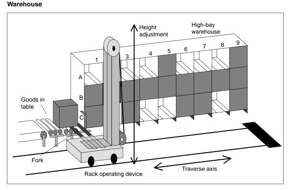
Figure 1-3 Example of a High-Bay Warehouse
