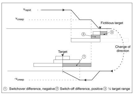
Figure 9-4 Loop Traverse to a Target at the Software Limit Switch End
