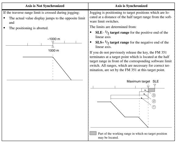
(1) Switchover difference positive (2) Switch-off difference positive (3) <sup>1</sup>/<sub>2</sub> target range
