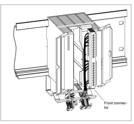
Figure 4-7 Wiring of the Front Connector
