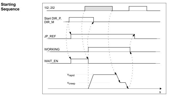
Figure 9-2 Starting a Seek-Reference-Point Traverse
