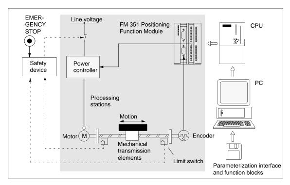
Figure 1-4 Electronic Cam Controller
