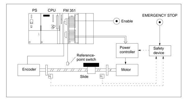
Figure 4-1 Wiring Diagram for an Open-Loop Positioning System
