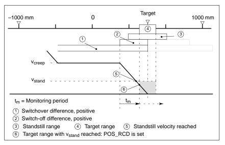
Figure 2-4 Target Approach of Positioning
